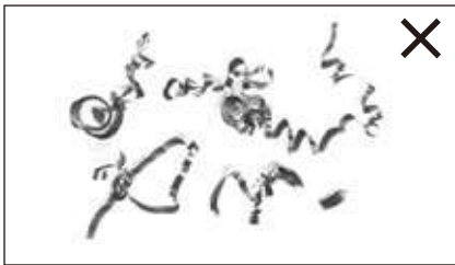
Apple-peel-like chips (Without curling)
