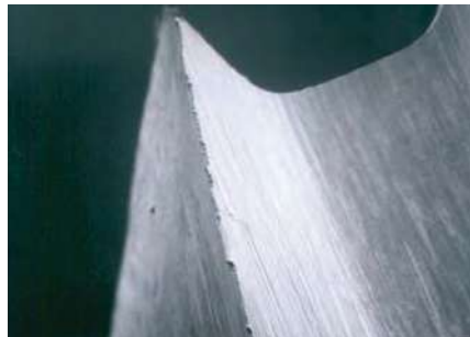
Surface of a conventional fluteless tap
