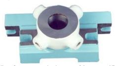
The quick acting collect fixtures standard range of 3 mm to 25 mm. fixture can be used for mass production in milling machine, drilling machines etc. The most common standard A25 collet is used in this fixture. It can be used vertically and horizontally.
