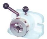
The A42 indexing fixture is a collet fixture with 12 equal dividing facility. It can be used vertically and horziontally. A42 collets can be used in this fixture. A simple lever operating mechanism is provided for indexing.
